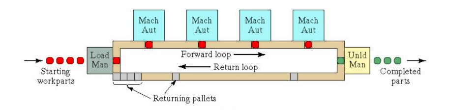
Rectangular layout allows recirculation of pallets back to the first station in the sequence after unloading at the final station
