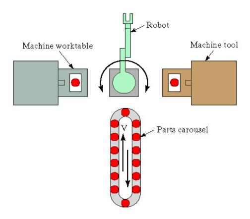
Automated manufacturing cell with two machine tools and robot. Is it a flexible cell?
