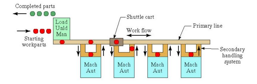
Linear transfer system with secondary parts handling system at each workstation to facilitate flow in two directions
